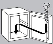
GB The safe must be anchored before being used.
